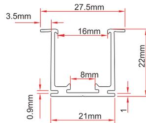
Note: Unless otherwise stated, the tolerance of the profile is  $\pm 0.5$ mm.
