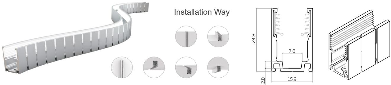
Note: Unless otherwise stated, the tolerance of the profile is  $\pm 0,2$  mm.
