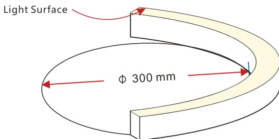
The light can only be bent along the light surface. Do not bend smaller than allowed minimum bend diameter.
