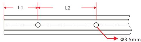
Note: Unless otherwise stated, the tolerance of the profile is  $\pm 0.5\text{mm}$ .
